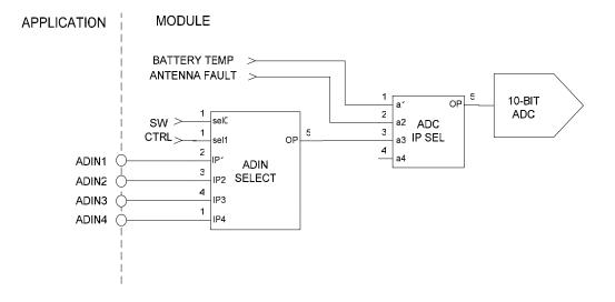
Figure 5.18-1 ADC sharing arrangement
